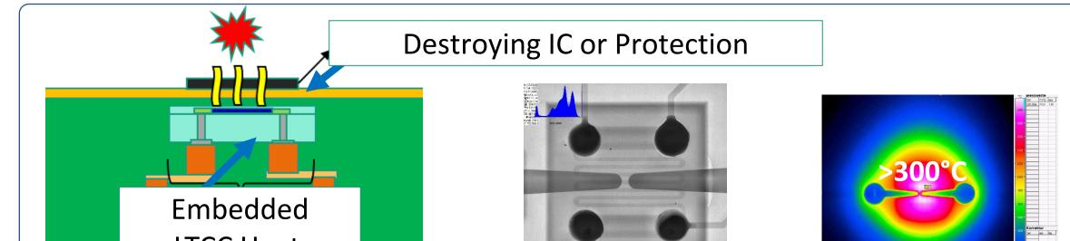
• The meander-shaped heater in LTCC can be placed near or under the IC to protect and influence or destroy the semiconductor ( $\Delta T > 250$  K) or the PCB.
